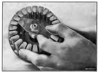
Fig. 13. Assembling a Sectional Armature Disk Punch
